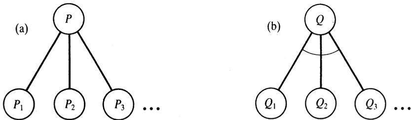
**Figure 13.3** (a) To Solve  $P$  solve any of  $P_1$  or  $P_2$  or... (b) To solve  $Q$  solve all  $Q_1$  and  $Q_2$ ...
