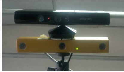
Fig. 3. Kinect and BumblebeeXB3 setup
