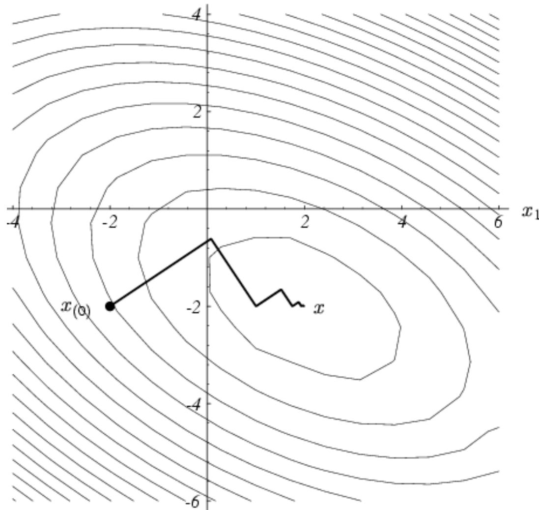
It has good performance in the initial stage of the iterative process. Converge very slow with a linear rate.
